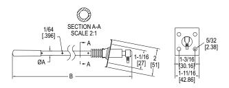
The Series AFG Averaging Flow Grid is a fundamental pressure-sensing device designed to sense velocity pressure in an air duct. When this output is connected to a suitable measuring instrument (i.e. manometer, pressure transducer, etc.) it may be used to determine air velocity or air flow rate.
